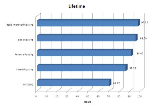
The next stage in the study was proposing improvements over the routing strategy to increase network's lifetime. In addition, a BMAC implementation for micaZ [6], which makes possible to sleep the nodes in order to make the routing protocol more power-efficient, was available for our researches.
