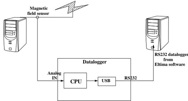
Figure 4: Energy Consumption: diagram of energy measurement device.
